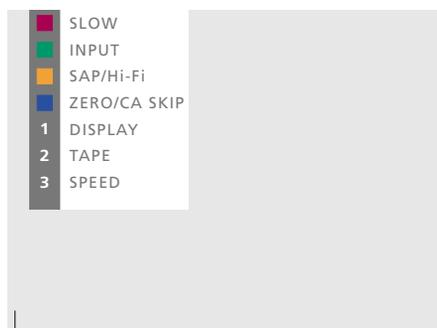
The menu overlay is an example of the menu overlay for a VCR. Via the Beo4 remote control, you can now operate the functions on the menu overlay. The functions you activate via the coloured Beo4 buttons can be activated directly, without calling up this menu overlay first.
